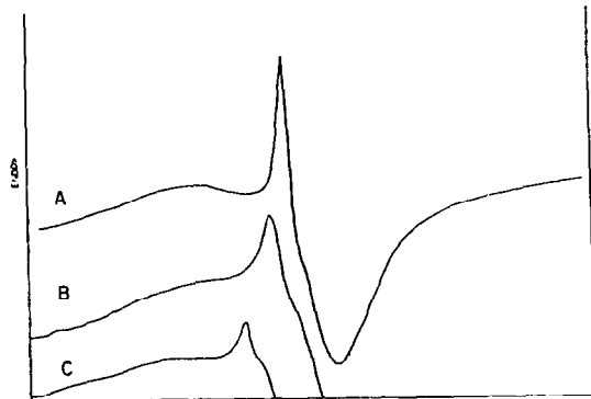
Fig. 6 DSC thermogram of Polyester partially oriented yarns with different finishes: A-deionized water. B-PEG 540. C-PEG 400.
